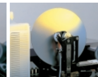
Back side periphery macro inspection (using a fiber optic illuminator)
